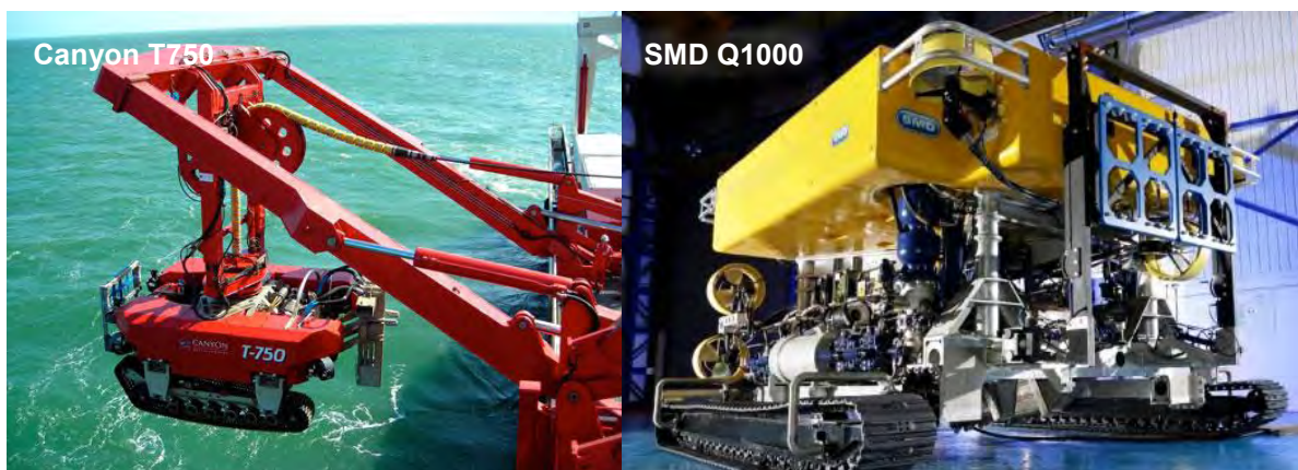
Figure 55 Example Power Cable Jetting ROVs
